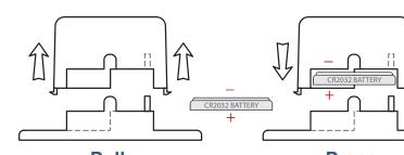
Pull (sensor away from base) Press (sensor back into base)
