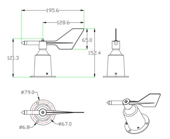
Please note that the arrow of the wind direction sensor points to true north during installation.
