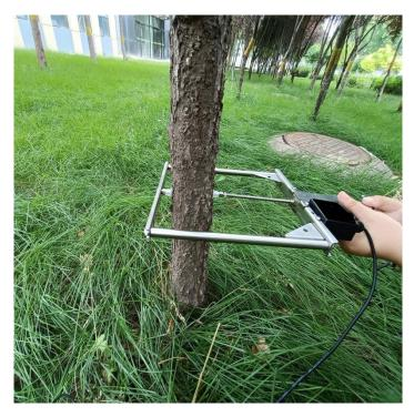
The third step is to penetrate four fixing holes with iron wire and fix them on trees or fruits, or fix them with brackets to keep the sensor balanced. (As shown in the following figure)
