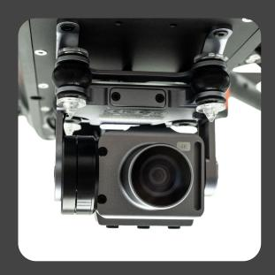
The Fisherman Max advanced version is pre-installed with a waterproof stabilized 4K camera for shooting smooth detail-rich footage. The lens can be tilt up and down via the remote controller, allowing you to see when and where the bait is released.
