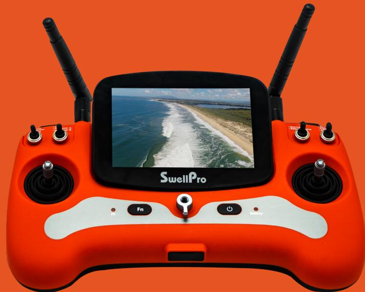
The advanced remote controller has an inbuilt multi-color display that can show the drone's live footage in 720P.
