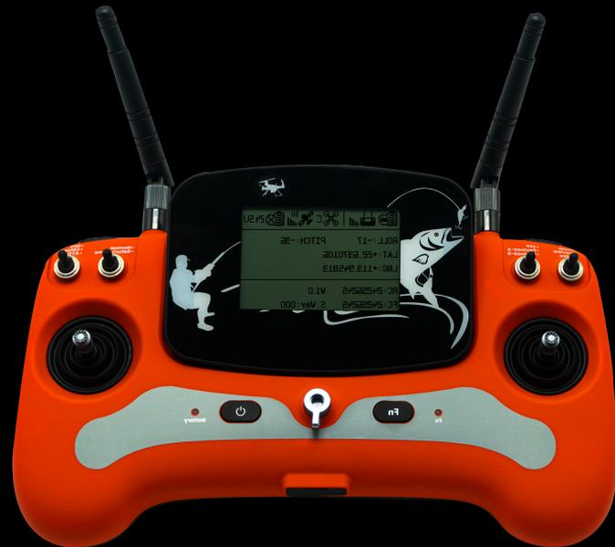
The basic remote controller has an inbuilt monochrome display that only shows flight telemetry.
